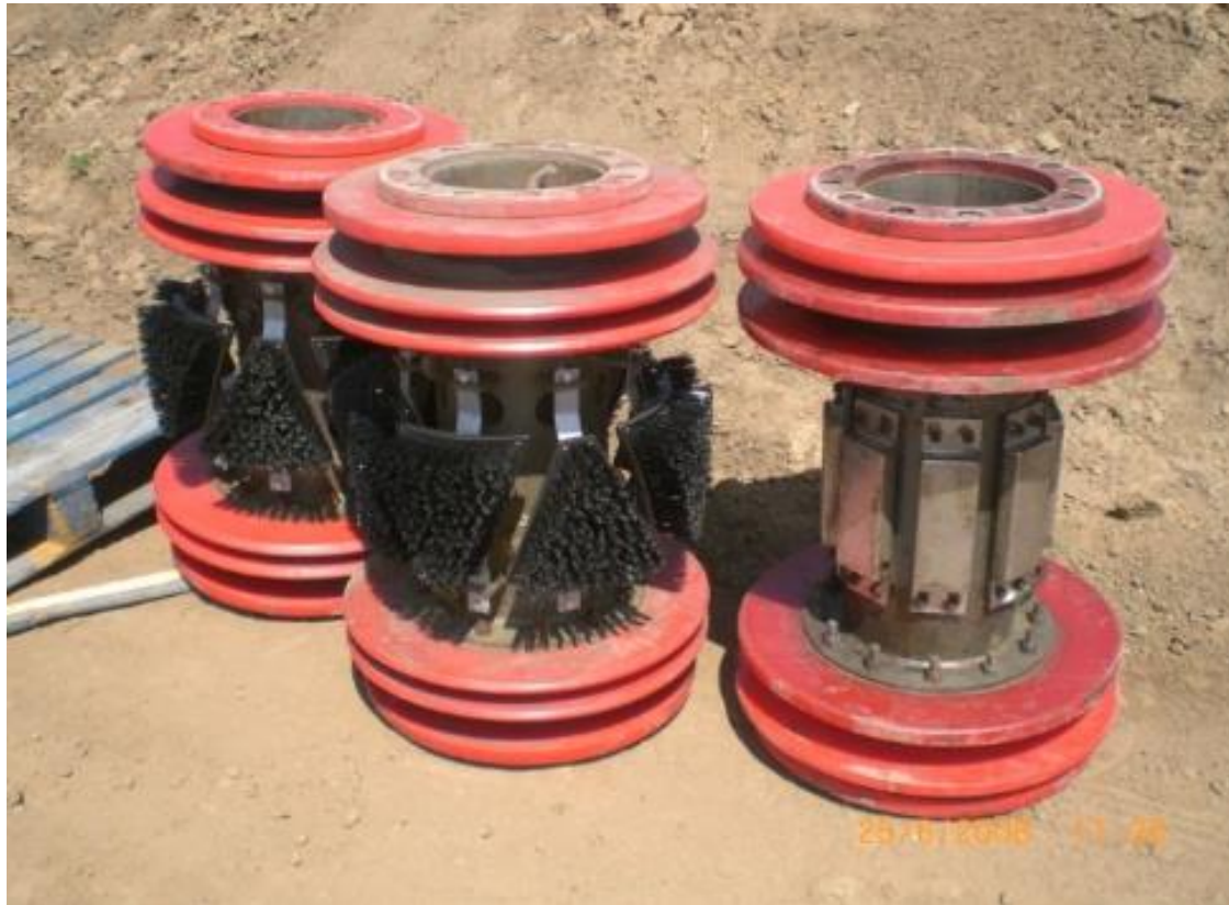
Figure 3-38: Variety of Cleaning Pigs (Brushes and Magnetic)
